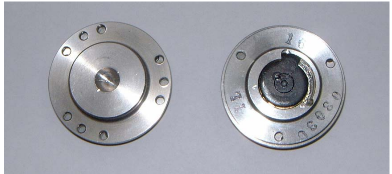
Left: three holes to adjust angle. Right: stopper at back side of core (screw position)
